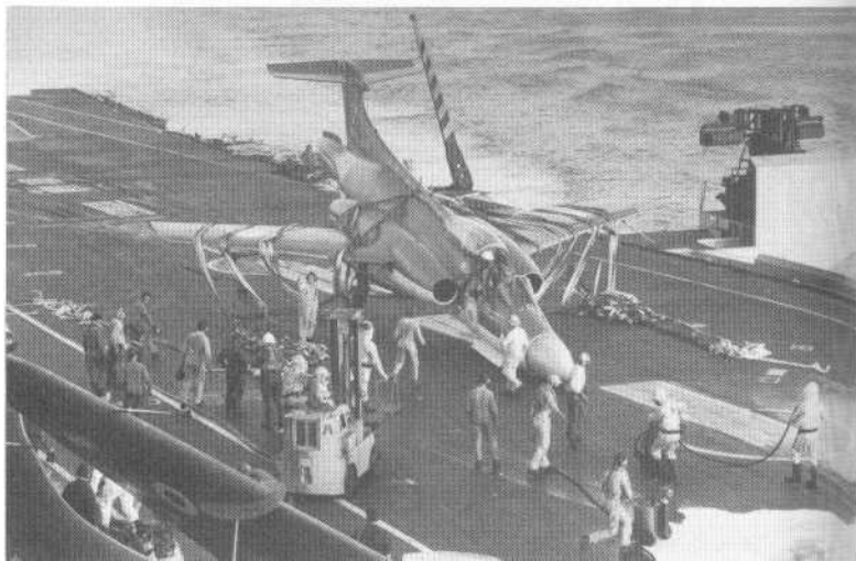
The arrested Buccaneer subsides gently onto its nose. The fire and rescue crews are not needed.
