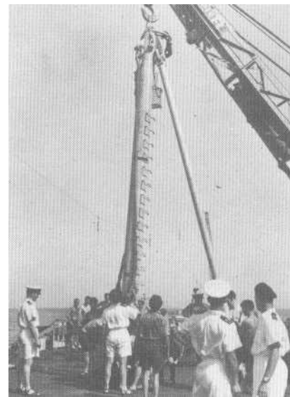
Stump mast for one of the 18 RAS's with R.F.A. RELIANT.
