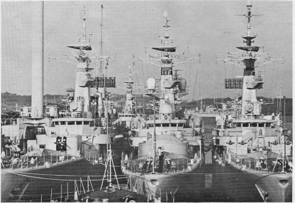
Not all Leanders look alike. This trio at Devonport are, from left to right, Scylla with 4.5 gun turret, Euryalus with Ikara missile system and Cleopatra with Exocet missiles (before launcher-containers were fitted).
