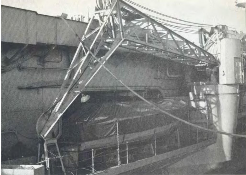
Principal task of the versatile ship's crane is loading supplies which may vary from sacks of flour to heavy spares - and stowed beside it - a 35 ft medium speed power launch
