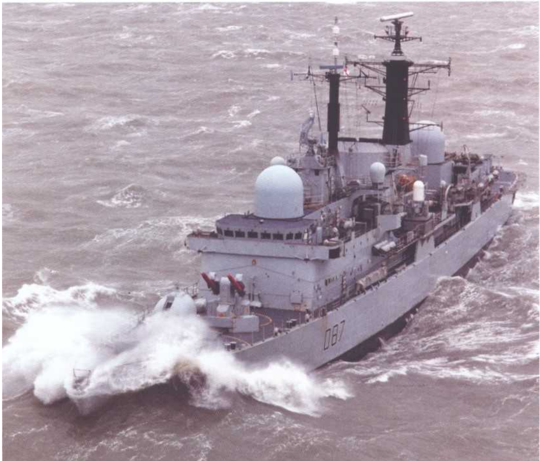
HMS NEWCASTLE at sea in the English Channel. Changes in appearance include the fitting of Type 1022 radar, Phalanx Close In Weapons System, a jammer and other close-range guns
