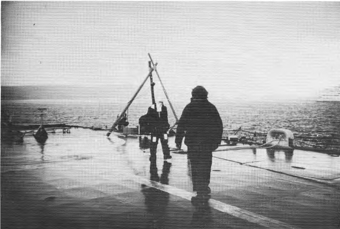
The sheerlegs being rigged to lift the bomb up to the flight deck. The amphibious shipping can be seen in the background in San Carlos Water.
