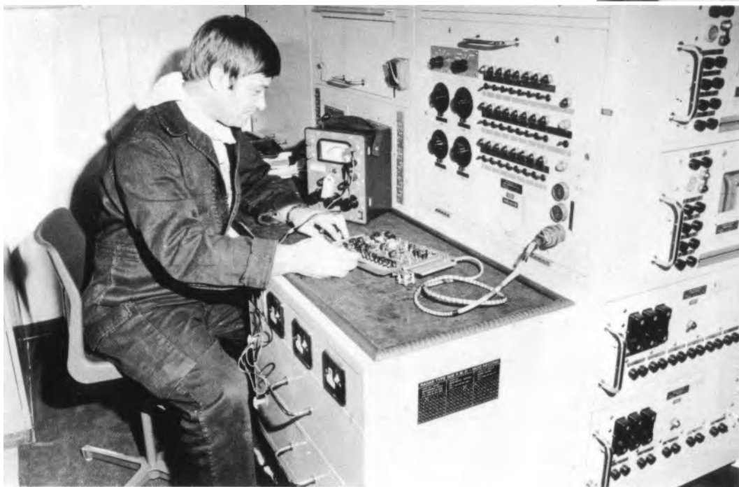
L.W.E.M. Galer — Repairing Printed Circuit Boards on the E. M.O. in the 909 Radar Maintenance Office.
