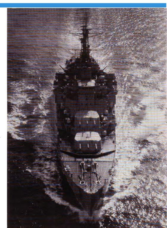
Sheffield was the first warship to carry 6" guns mounted in triple turrets, two forward and two aft. She was capable of maintaining a succession of 23-gun broadsides with a total output of 96 rounds per minute.
